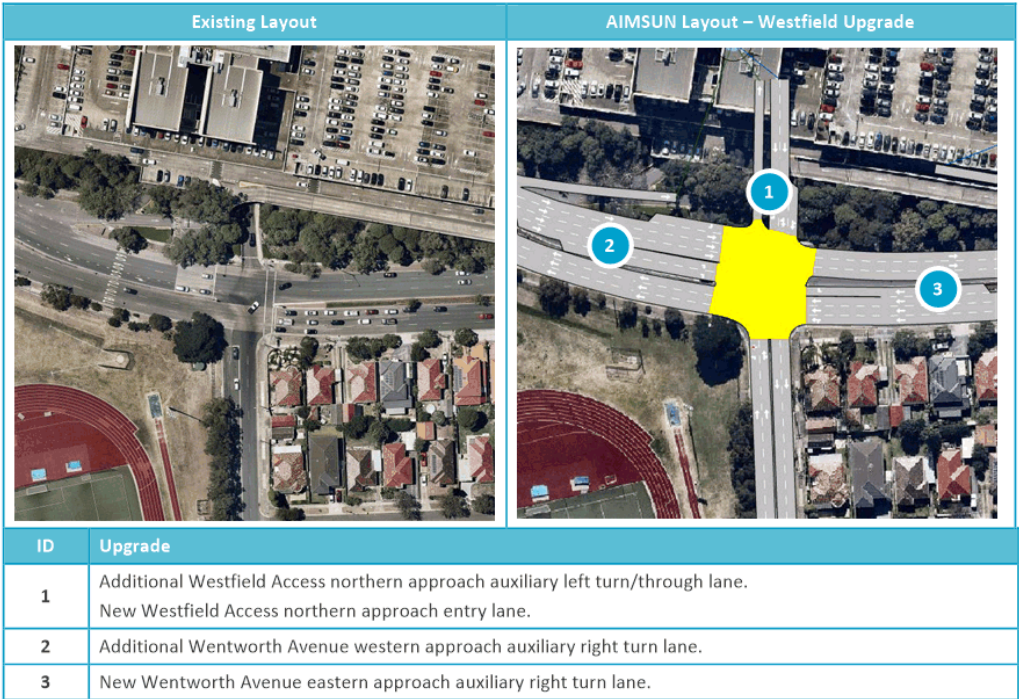
Figure 11 Existing and Proposed Layout: Wentworth Avenue/Denison Street/Westfield Access Intersection
