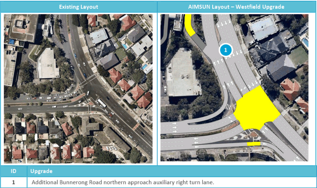
Figure 12 Existing and Proposed Layout: Wentworth Avenue/Bunnerong Road Intersection
