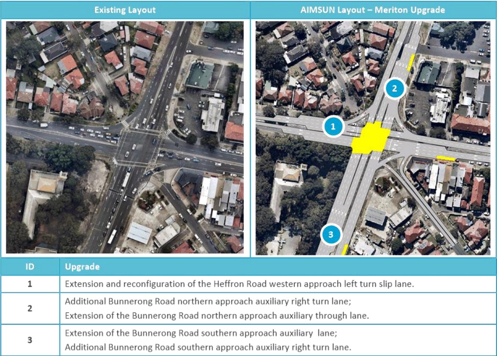
Figure 4 Existing and Proposed Layout: Bunnerong Road/Heffron Road/Maroubra Road Intersection
